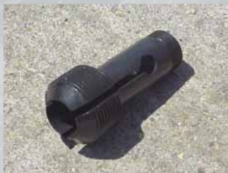
Typical Flow Activated Releasable Fishing/Bulldog Spear Slip
